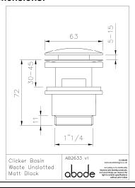
• Product mounted where: Surface • Recommended hole size: Ø 43-55 mm
